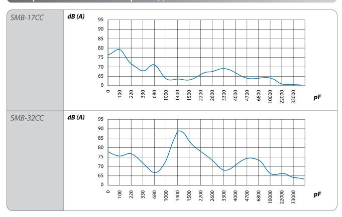
All measurements are made in free air @ 21 °C @ 30 cm @ 12 Vdc.
