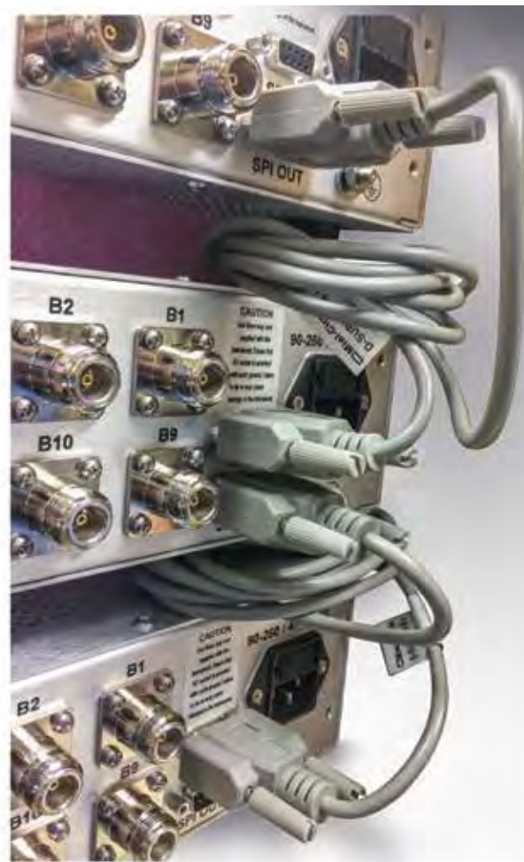
3 ZTDAT racks “daisy chained” via SPI ports
